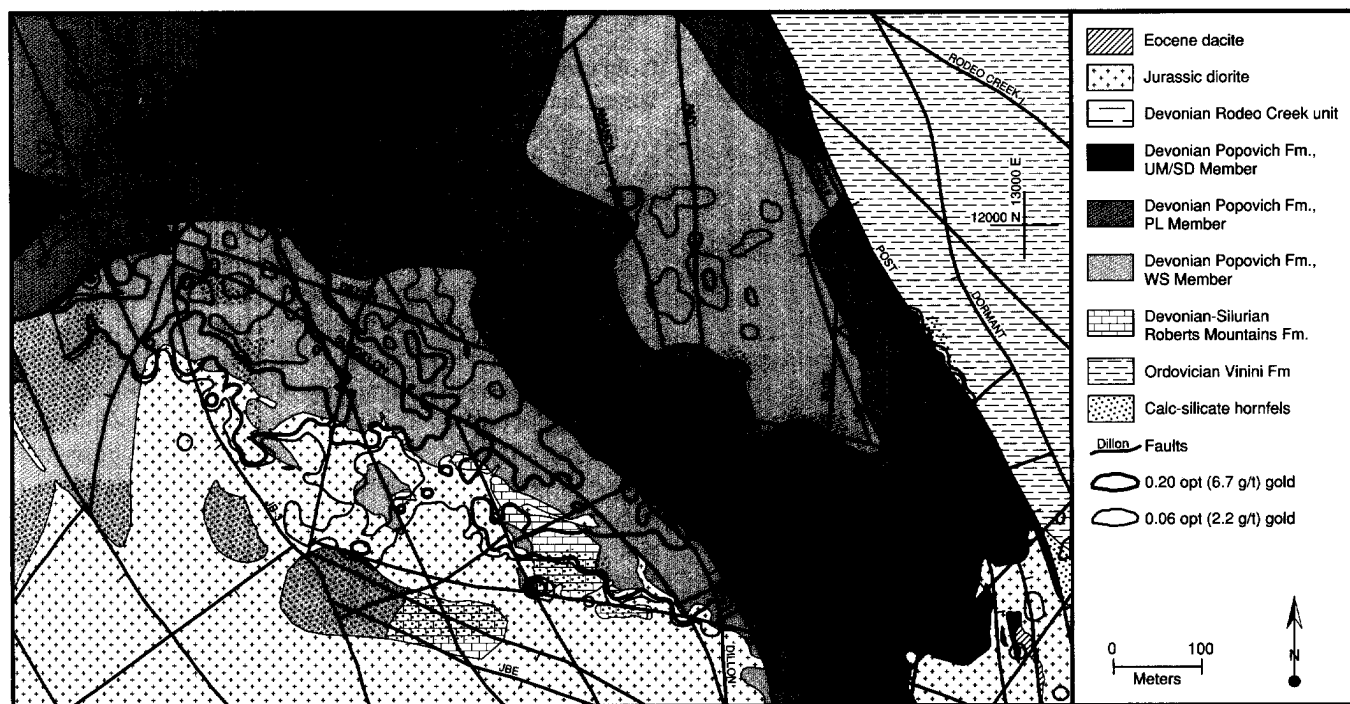
Figure E-9. Level plan at the 4700 level (1,433 m) of the Betze and Deep Post subdeposits of the Betze-Post deposit. Important ore controls shown at this level are the Wispy Member of the Popovich Formation, the Dillon fault zone, and the contact of the Jurassic diorite. Small displacements on faults are not shown. The location of the level plan is shown in figure E-5.
